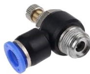
SL0602-1/4" BSP MALE THREAD SWIVEL 90 DEGREE WITH SPEED ADJUSTER TO TUBE 6MM
