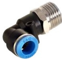
PL0802-1/4" BSP MALE THREAD 90 DEGREE ELBOW TO 8MM TUBE
