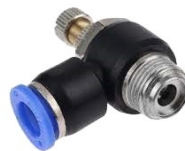
SL1202-1/4" BSP MALE THREAD SWIVEL 90 DEGREE WITH SPEED ADJUSTER TO TUBE 12MM
