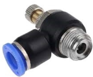
SL0601-1/8" BSP MALE THREAD SWIVEL 90 DEGREE WITH SPEED ADJUSTER TO TUBE 6MM
